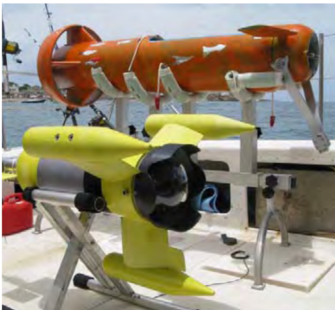
Jonas is the red one, Simeon is yellow. Developed with the French Navy, these underwater camera drones are tethered to the mother ship with a fiber optic cable. Photos: Alexandre Bügel.
