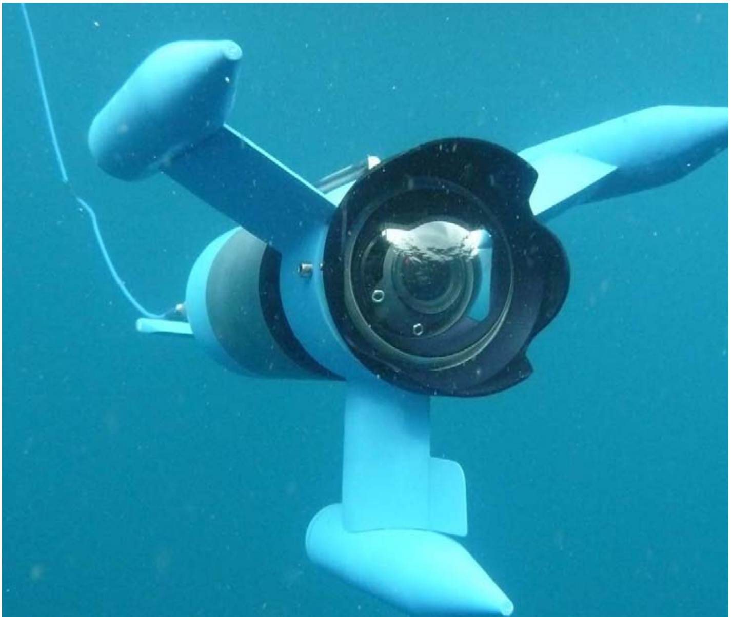
Jonas is the red one, Simeon is yellow. Developed with the French Navy, these underwater camera drones are tethered to the mother ship with a fiber optic cable. Photos: Alexandre Bügel.
